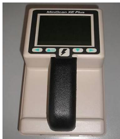
**Slika 11** Kolorimetar Hunter-Lab Mini ScanXE
