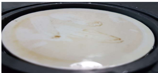
Fig.5. Clogging on the surface
