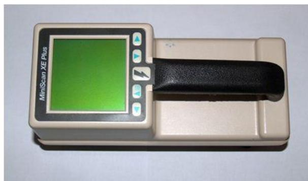
**Slika 20** Hunter- Lab Mini ScanX
