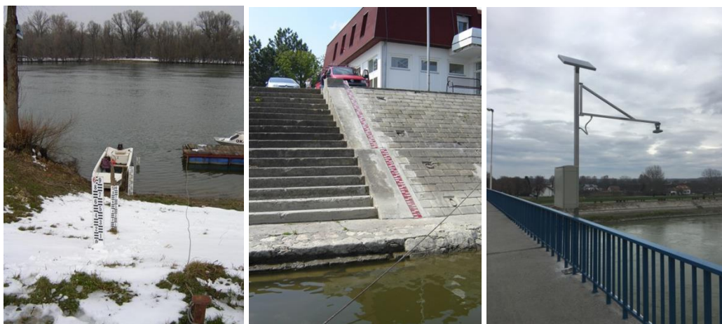
Slika 1. Opažanje vodostaja - običnom letvom, kosom u obaloutvrđi i elektronički, prikladnim senzorom Figure 1. Water level observation - by water level measurement stock (vertical or on the slope of river embankment) and electronically, with a suitable sensor
