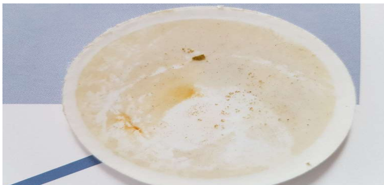
Fig. 8. Deposits on the membrane surface after filtration
