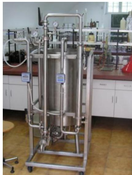
Slika 6 Membranski filter (Web 6)
