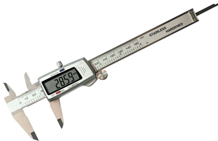
Slika 5: Šubler (Izvor: https://bit.ly/3wie4eq )
