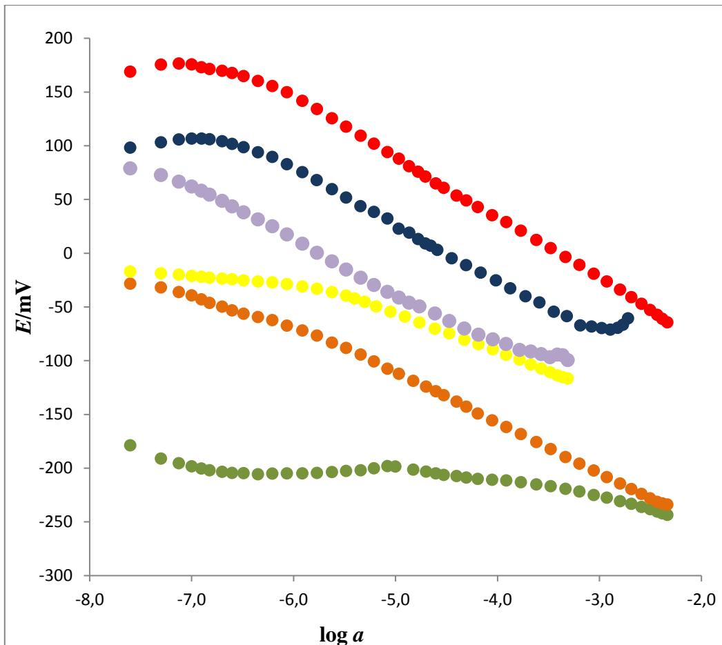
Slika 20. Usporedba odziva MWCNT-TODA-TPB elektrode na  $\bullet$  NaDDS,  $\bullet$  NaDBS,  $\bullet$   $\text{C}_{14}\text{H}_{27}\text{NaO}_3\text{S}$ ,  $\bullet$   $\text{C}_{12}\text{H}_{25}\text{NaO}_3\text{S}$ ,  $\bullet$   $\text{C}_{10}\text{H}_{21}\text{NaO}_3\text{S}$  i  $\bullet$   $\text{C}_8\text{H}_{17}\text{NaO}_3\text{S}$  u vodi
