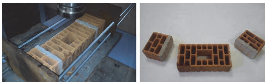
Figure 4. Mortar head joint sliding failure
