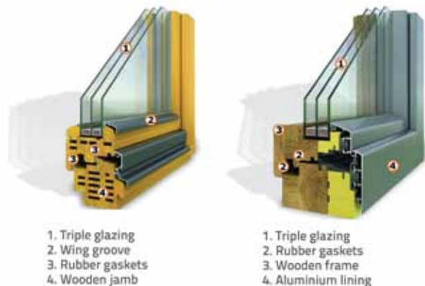
Figure 15. Detail of a wooden window with triple glazing: a) without frame thermal protection; b) with frame thermal protection
