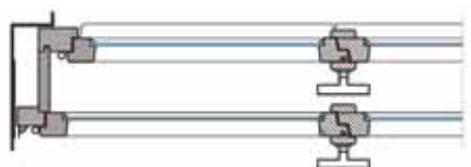
Figure 10. Horizontal cross-section of double double-sash window
