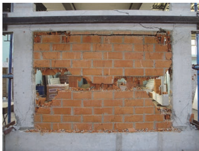
Figure 6. Failure of masonry infill walls made with hollow clay units (specimens O1_{bpm} and O3_{bpm} )
