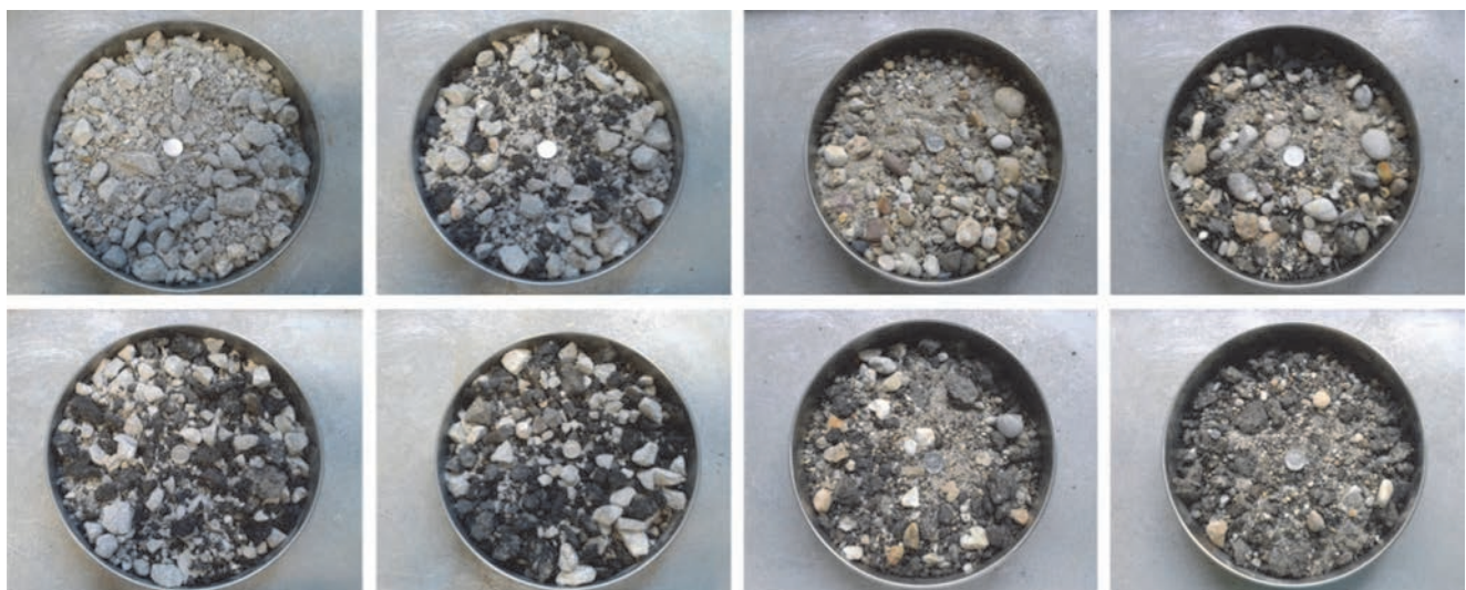
Figure 2. Recycled asphalt mixed with limestone (left) and gravel (right)
