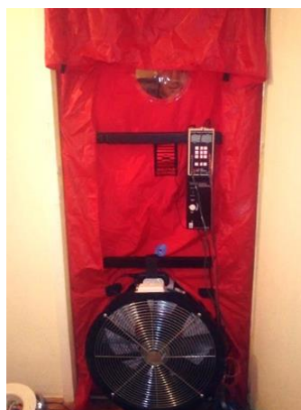
Figure 3 Blower door fan with manometer DG-700 [10]
