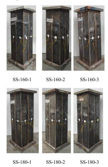
Fig. 9. Failure modes of test CFDSST columns with varying concrete strengths  $f_c$ .
