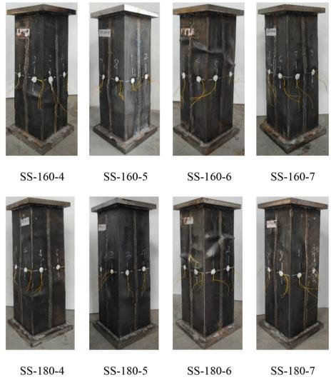
**Fig. 10.** Failure modes of test CFDSST columns with varying values of  $t_0$  or B.
