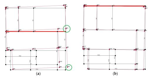
Figure 10. Eigen modes. (a) First eigen mode, Y-direction; (b) second eigen mode, X-direction.
