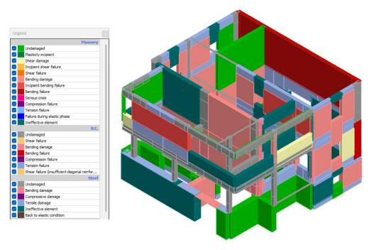
Figure 13. Damage of the structure during analysis No. 23.
