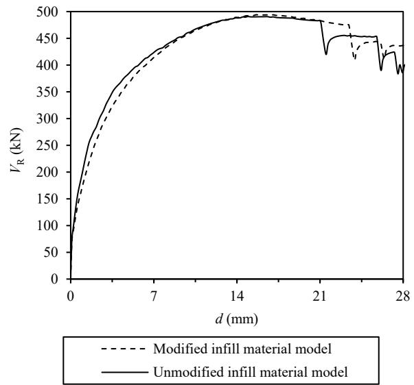
Figure 10 Force displacement diagram of infilled frame model
