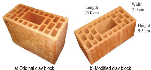
Figure 1 Masonry unit
