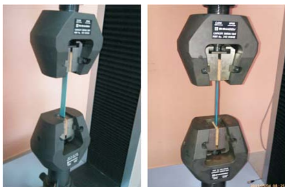
Figure 2 Testing machine and multiple strap samples
