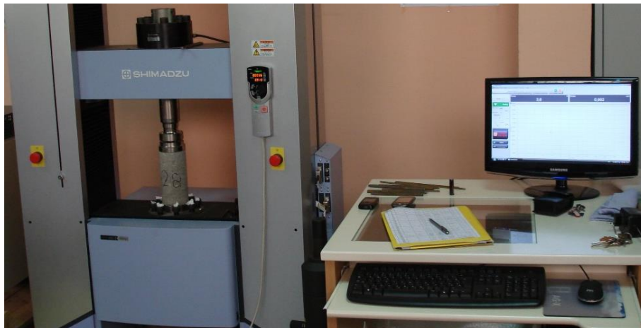
Figure 3 Equipment used to test compressive strength
