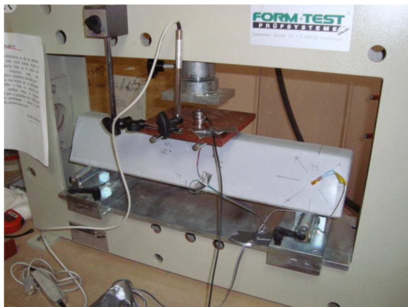
Figure 3. Test rig for fiber-reinforced polymer beams
