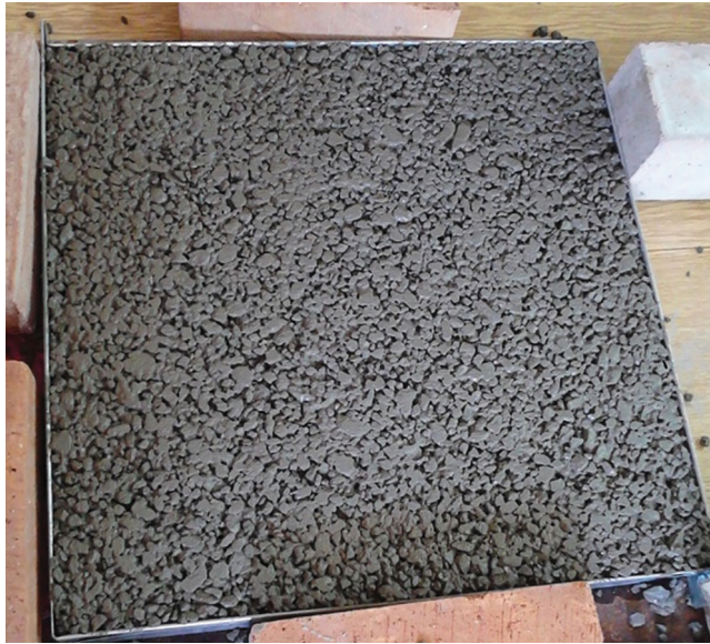
Figure 3. Pervious concrete slab for sound spectral analyses.
