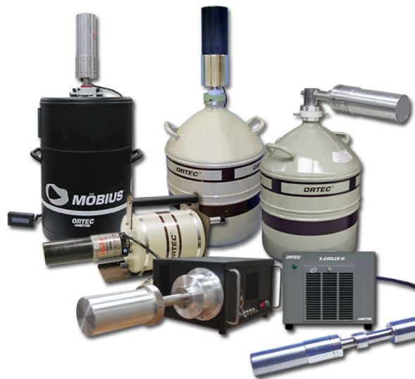
Figure 3.2.4: HPGe semiconductor detector [21].
