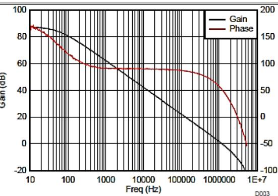
Figure 3. Error Amplifier Open-Loop Gain and Phase vs Frequency,  $V_{CC} = 15$  V,  $R_L = 100$  k $\Omega$ , and  $T_A = 25$  °C
