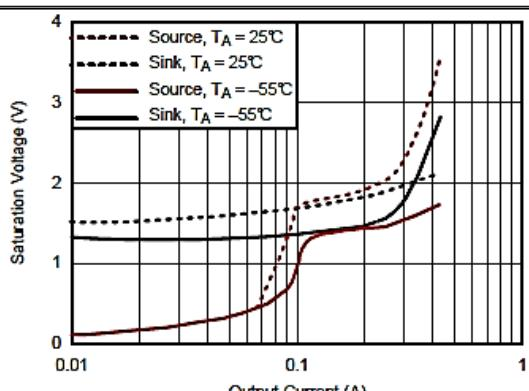
Figure 8. Output Saturation
