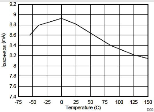
Figure 1. Oscillator Discharge Current vs Temperature for  $V_{CC} = 15$  V and  $V_{osc} = 2$  V
