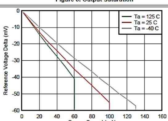
Figure 6. VREF Voltage vs Source Current
