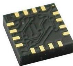
Sl. 3.16. Magnetometar HMC5883L. [Izvor: https://www.sparkfun.com ]
