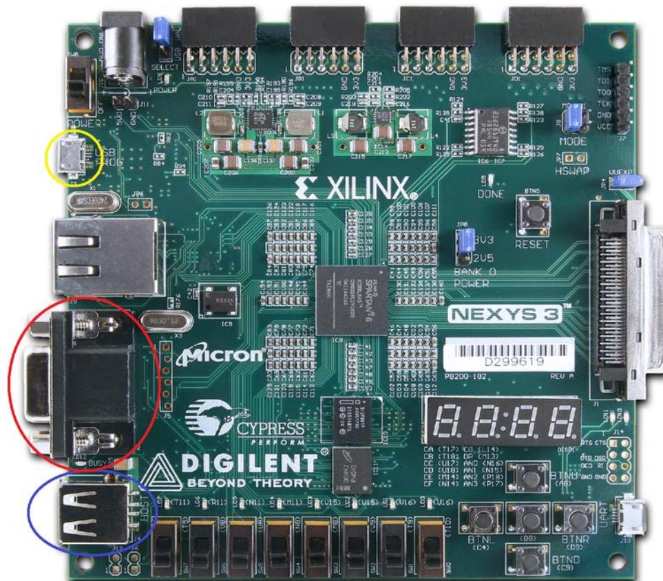
Slika 4.1: Nexys 3 Spartan 6 FPGA Board [9].
