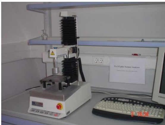
Slika 7 TA.XT2 Plus Texture Analyser (Tanasković, 2014)
