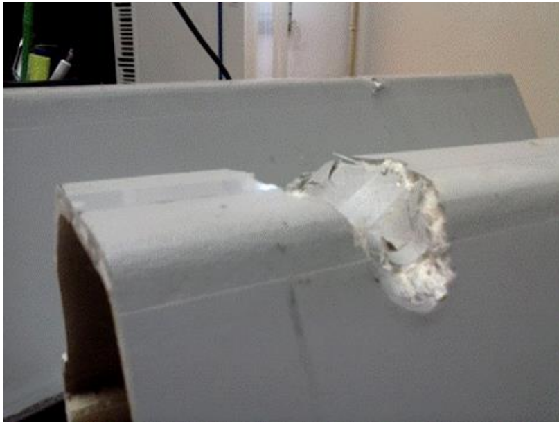
Figure 2 Local beam deformation [4]
