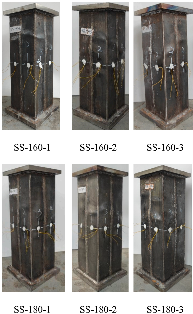
Fig. 9. Failure modes of test CFDSST columns with varying concrete strengths f_c .
