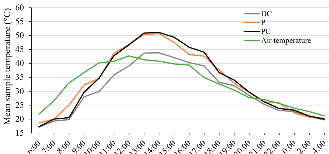
Figure 7. Concrete pavement surface temperature change on grass base.
