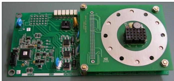
Slika 3-6 SCEM modul; Switchgear Cable Entry Module
